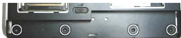
Fig. 9 Removing the touchpad assembly screws
